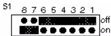
Figure 13: S1 has eight dip switch positions. (Lettering inverted for this illustration.)
